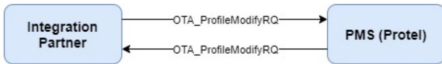
To stop this endless loop, we have implemented the "Caused-By CorrelationID". The "Caused-By CorrelationID" is automatically added to the outbound messages by the PMS if a modification has been made due to an inbound message. Based on the "Caused-By CorrelationID", our ESB knows to which Ontegration Partner the message does not have to be sent.
